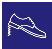
Assorbimento energia al tallone Energy absorption at the seat region
